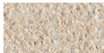
bocciardato / bush-hammered / gestockt
