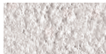
bocciardato / bush-hammered / gestockt
